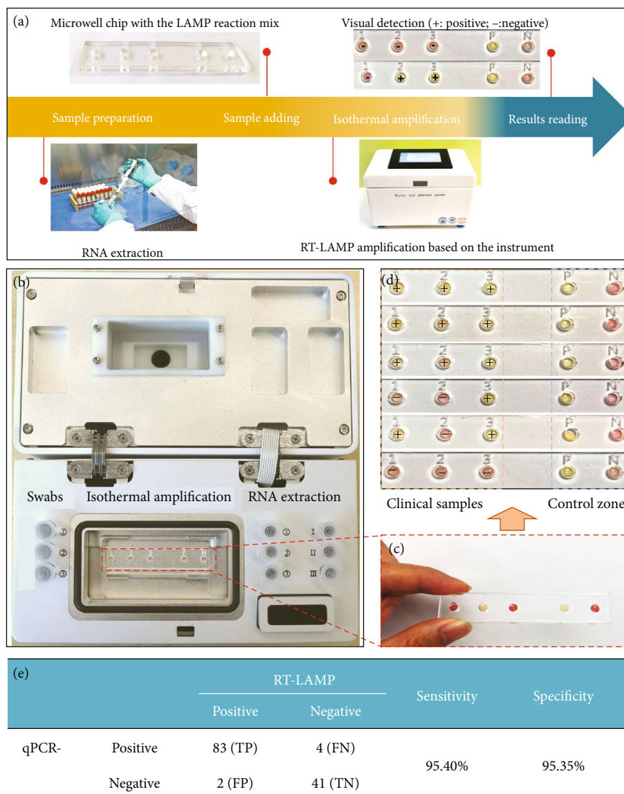
FIGURE 4: Clinical validation of the RT-LAMP detection platform with the real samples of COVID-19 patients from the West China Hospital, Chengdu. (a) The detection process using our platform, including RNA extraction, amplification, and results reading. (b) Photographs of the microwell chip mounted on the platform prior to the addition of RT-LAMP buffer and clinical samples. (c) The color in microwell changes from pink to yellow with positive samples. (d) Detection results of clinical samples on the microwell array. (e) The diagnostic accuracy for the clinical samples based on our platform against reference laboratory diagnosis (compared with RT-qPCR as a benchmark), based on a total of 130 clinical samples (87 COVID-19 positive and 43 negative).
