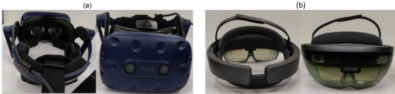
Figure 2. Example of VST and OST devices. (a) HTC VIVE with occluded display. (b) Microsoft HoloLens with transparent display.
