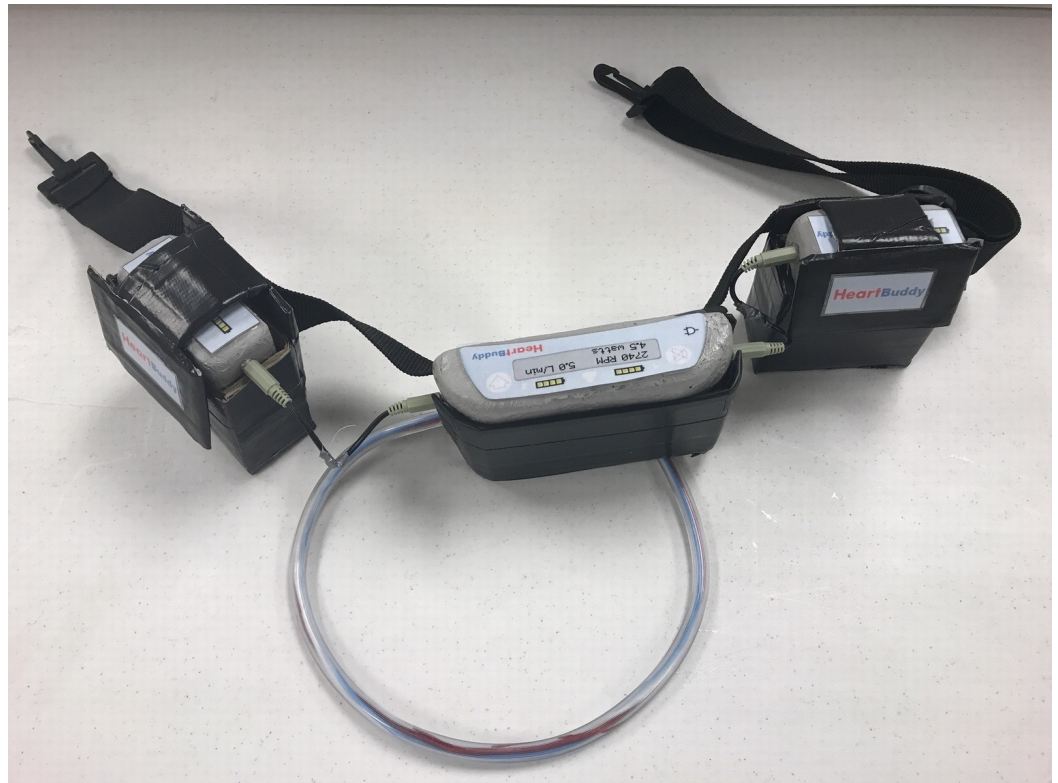
FIGURE 3: Final simulated left ventricular assist device (LVAD) as per the materials listed in Figure 1 and replication instructions
