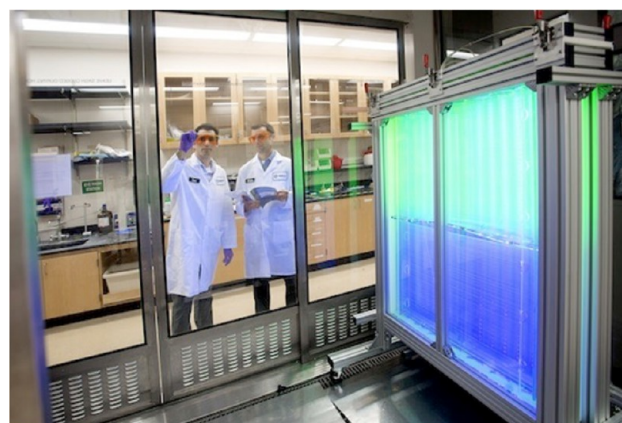
Figure 4. Process-scale photoredox flow reactor at Merck. Photo courtesy of Merck and Co. Inc. Copyright 2016 American Chemical Society. 168
