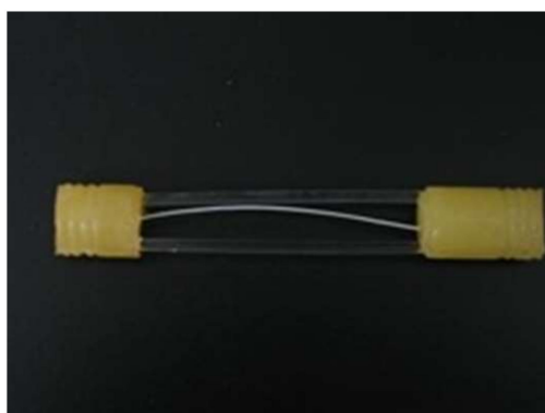
Figure 4. Photograph of a hollow fiber membrane module prepared in this study.
