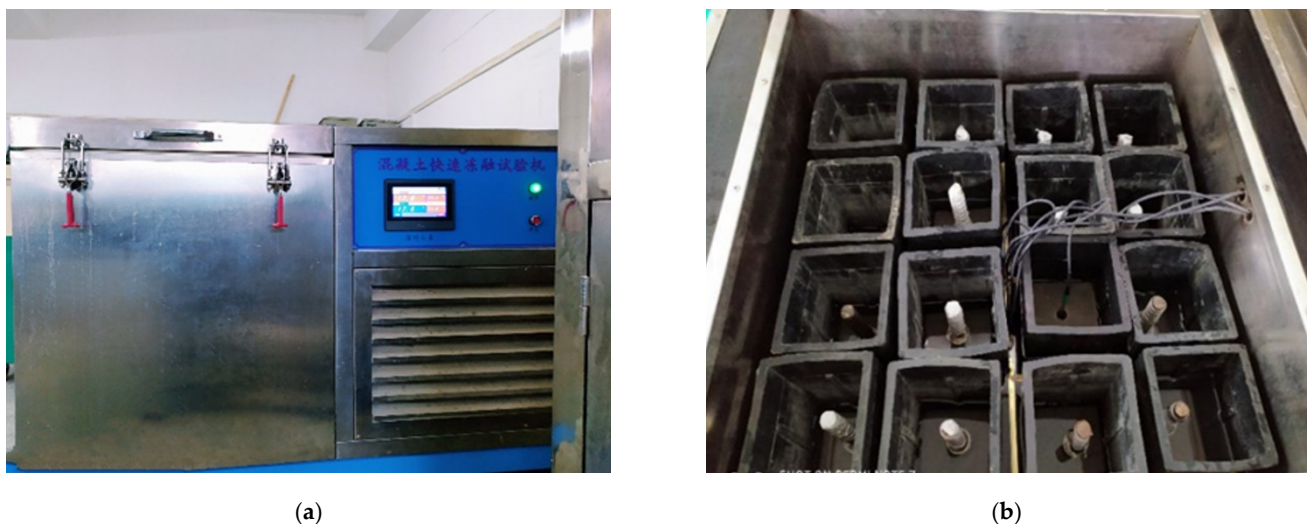
Figure 2. Freeze–thaw method: (a) Instrument; (b) Internal configuration.
