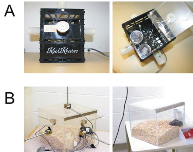
Fig 1. Diagram of the EMF exposure apparatus. A. In vitro exposure device is 12 cm on each side and fitted with 6 solenoids, one on each face of the cube, which are all activated during Thomas-EMF exposures. Plates containing cells are placed inside the cube for exposure. For the sham condition, the cells are placed in the box but electrical pulses are not sent to the solenoids. B. In vivo exposure device is 30 cm on each side and fitted with 6 solenoids, one on each face of the cube, and all solenoids are activated during Thomas-EMF exposure. The control box is not fitted with solenoids. A group of 5 mice is placed in the box for the exposure period.
