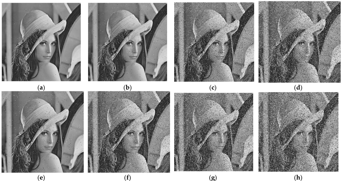
**Figure 11.** Noise attack test. (a–d) with salt-and-pepper noise densities of 0.001, 0.01, 0.05, 0.1, respectively; (e–h) with Gaussian white noise variance values of 0.2, 0.3, 0.4, 0.5 respectively.
