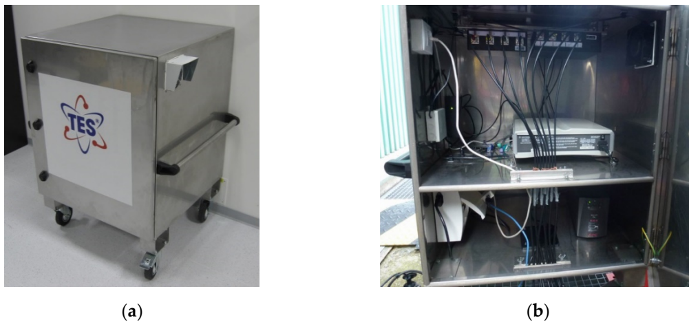
Figure 7. The main unit of the PD UHF diagnostic system: closed (a) and open (b) case views.
