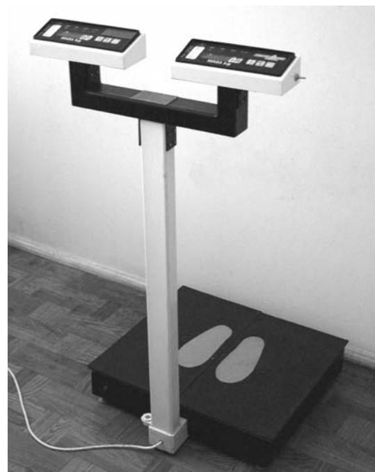
Figure 3. Electronic balance specially constructed for this research
