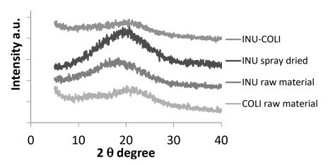
**Figure A1.** PXRD patterns of the formulations and raw materials. XRD measurements were conducted on samples placed in a low background silicon holder, using a Rigaku Miniflex II desktop X-ray diffractometer (Rigaku, Tokyo, Japan). The samples were scanned over a range of 5–40°  $2\theta$  at a step size of 0.05°/s.
