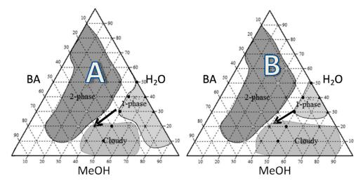
**Figure 1.** Butyl acetate–methanol–Water pseudoternary phase diagrams obtained in the presence of **(A)** inulin (INU) at  $0.75 \ w/w\%$  and, **(B)** a mix of INU at  $0.5 \ w/w\%$  and colistin (COLI)  $0.5 \ w/w\%$ . The arrow in the diagram indicates the relative change in solvent composition that should occur during the spray drying.
