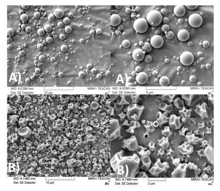
**Figure 2.** SEM micrographs of **(A)** spray-dried INU, **(B)** INU-COLI. The samples were coated with a 10 nm-thick gold film. Primary electrons were accelerated under a voltage of 5 kV. Images were formed from the collection of secondary electrons.
