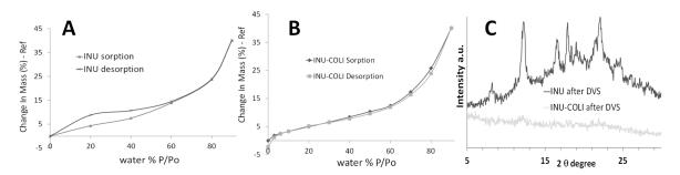
**Figure A2.** Water sorption–desorption isotherms obtained by DVS of **(A)** INU spray-dried powder and **(B)** INU-COLI spray-dried powder. **(C)** XRD patterns of INU and INU-COLI after one water sorption–desorption cycle.
