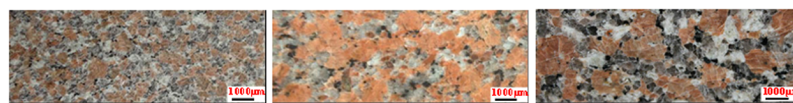
Fig 13. Granites with three kinds of grain sizes processed by digital image. (a) grain size = 1.01mm (b) grain size = 2.12mm (c) grain size = 3mm.
