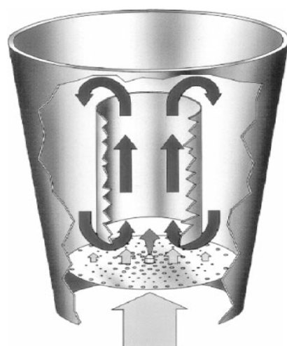
Figure 1. Diagram of bottom spray fluidized agglomerator (reprinted with permission from Glatt).
