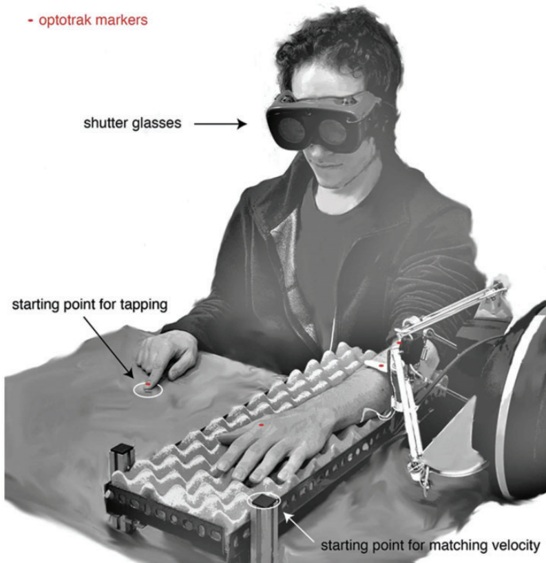
Figure 1. The experimental setup. Red dots indicate the position of the Optotrak markers, and white circles indicate the two starting points for the finger, one for the tapping movements of the Position and Interception experiments and the other for the movements in the Velocity experiment.
