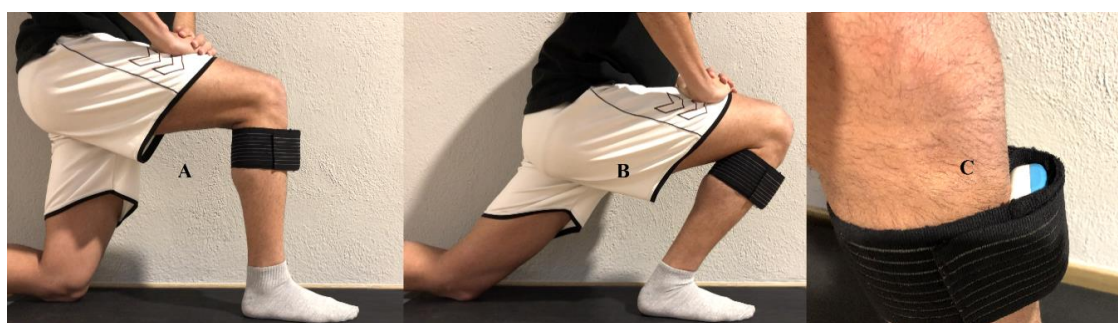
Figure 1. Athlete wearing a WIMU Pro device for the measurement of weight-bearing ankle dorsiflexion. (A) starting point of weight-bearing lunge test; (B) ending point of weight-bearing lunge test; (C) WIMU Pro device in touch with the tibia.
