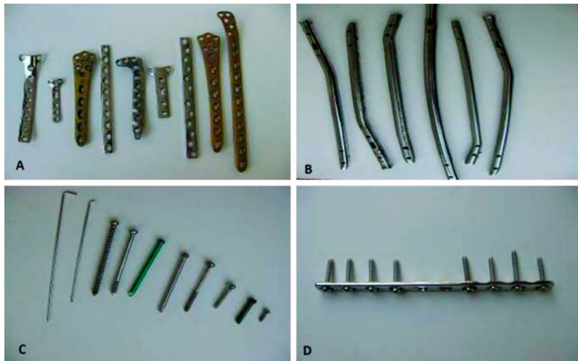
Figure 1. Different types of post-service metallic implants: (A) plates of stainless steel and titanium; (B) intramedullary nails of stainless steel; (C) screws and pins of stainless steel and titanium; (D) a plate with stainless steel screws [4].
