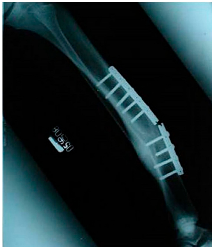
Figure 2. Radiographic image of a failed stainless steel implant due to fatigue [17].
