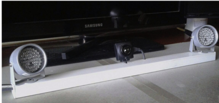
Fig. 1. Eye tracker hardware consisting of two infrared illuminators and camera.
