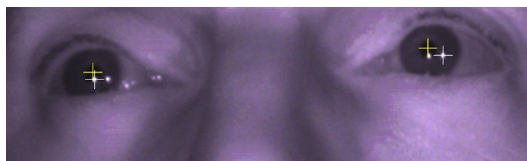
Fig. 6. A frame from the eye video that is linked with the gaze plot of raw data samples. The frame changes as the analyst scrolls through the timeline. The crosshairs show the reported centres of the pupils and corneal reflections.
