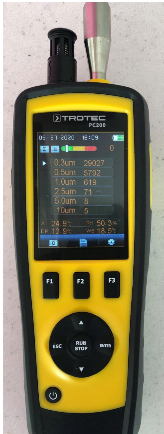
Figure 3. Particle sensor PC200 (Trotec GmbH, Schwerin, Germany) used in the experiment.
