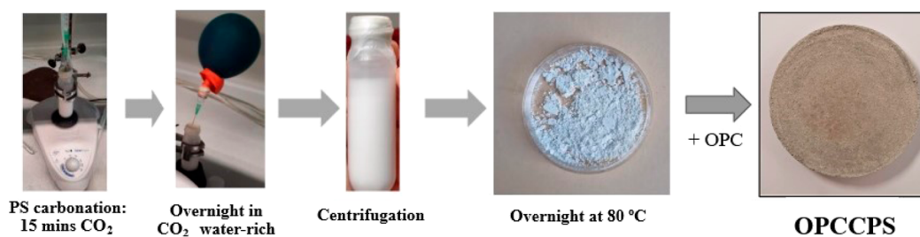
Figure 1. Overview of the experimental setup of carbonation of Periwinkle shell ash.
