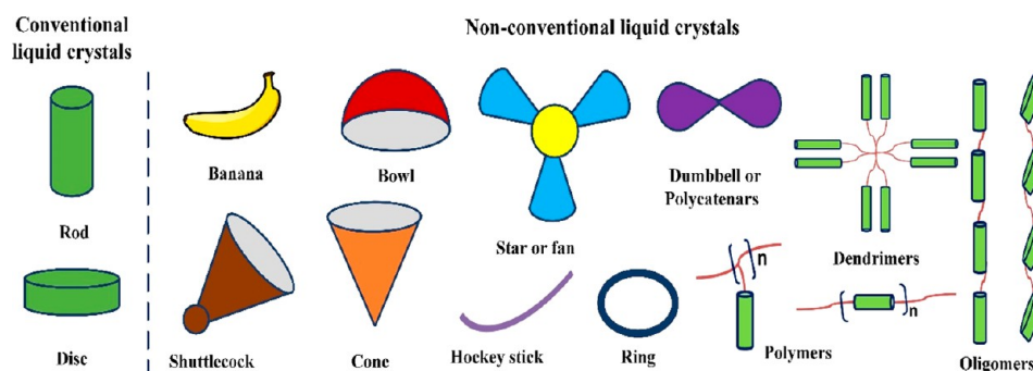
Figure 1. Schematic diagram showing conventional and nonconventional molecular shapes used for the stabilization of LC phases.
