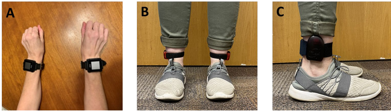
Figure 2. Wearable sensor placements for included studies. A) Participants in all studies wore ActiGraph GT3X+ or ActiGraph GT9X Link sensors on each wrist (picture shows Link sensors). B) Participants in three studies (Bailey et al., 2013, Waddell et al., 2017, and Bland et al., 2021) also wore bilateral ankle sensors (ActiGraph GT3X+). C) In one study (Lang et al., 2022), individuals with Parkinson’s disease and a subset of individuals with stroke wore a Modus StepWatch Activity Monitor (Modus Health LLC) on their less affected ankle.
