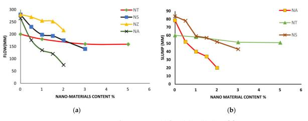
Figure 3. Impact of various NMs: (a) flowability; (b) slump [9].
