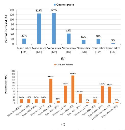
**Figure 7.** (a) Compressive strength in the presence of micro and nano silica particles [169]; (b) Compressive strength percentage increment for cement paste [82,125–130]; (c) Compressive strength percentage increment for cement mortar [170–180].
