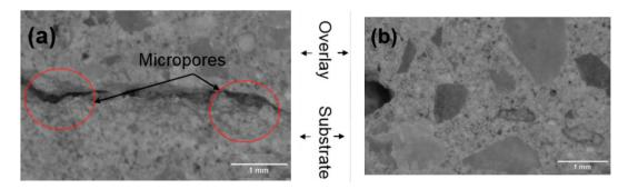
Figure 22. SEM images: (a) specimens with 0.5 wt% NC and (b) a control specimen [253].
