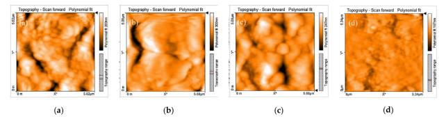
**Figure 16.** AFM analysis of concrete with: (**a**) plain cement; (**b**) nano-silica; (**c**) silica fume; (**d**) polypropylene fibers and nano-silica [181].
