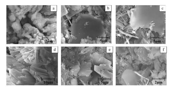
**Figure 18.** SEM of cement composites modified by different contents of GONPs: (**a**) no GONPs; (**b**) 0.01% GONPs; (**c**) 0.02% GONPs; (**d**) 0.03% GONPs; (**e**) 0.04% GONPs; (**f**) 0.05% GONPs [249].
