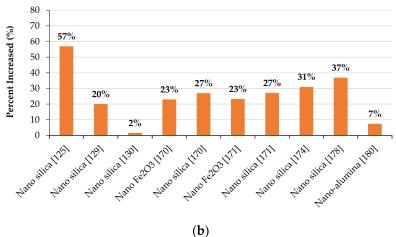
**Figure 10.** (a) MPC paste's flexural strength with different dosages of Fe<sub>2</sub>O<sub>3</sub> powder [28]; (b) Flexure strength percentage increment for cementitious composites [125,129,130,170,171,174,178,180].
