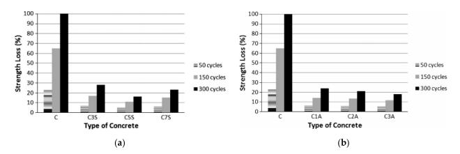
Figure 8. Strength loss of samples having: (a) NS; (b) NA [141].
