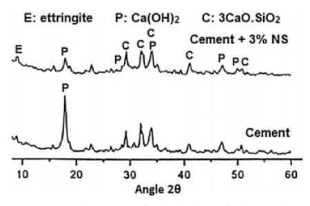
**Figure 5.** Interaction between NS and Ca(OH)<sub>2</sub> at the interface between the paste and the aggregate [126].
