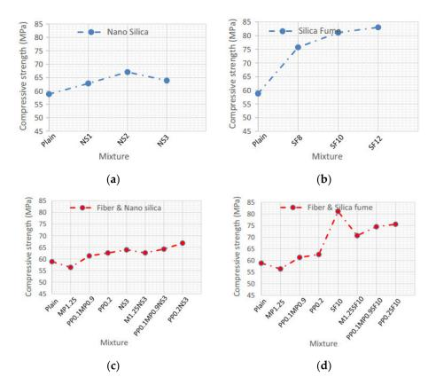
Figure 9. Compressive strength of concrete having: (a) NS; (b) SF; (c) fibers and NS; and (d) fibers and SF [181].
