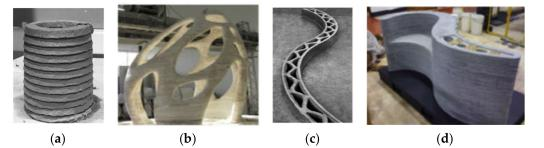
Figure 2. 3D printing: (a) 3D printed object [106]; (b) D-Shape; (c) Contour crafting; (d) Concrete printing [98].
