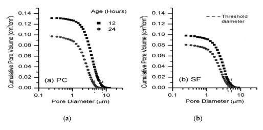
Figure 12. Coarse capillary pore size distributions at early ages: (a) Portland cement concrete; (b) SF concrete [210].
