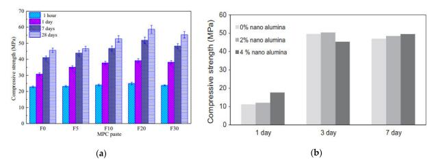
**Figure 6.** Compressive strength: (a) MPC paste varies with different dosages of Fe<sub>2</sub>O<sub>3</sub> powder [28]; (b) Cement replaced with 0%, 2%, and 4% of Nano-Al<sub>2</sub>O<sub>3</sub> [167].
