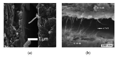
**Figure 20.** (a) C-NFs pulled out from a microcrack, and (b) bridging a crack by embedding CNTs in a cement-based composite [250].
