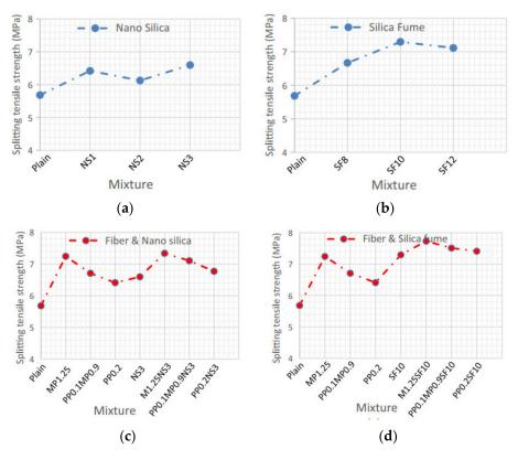
Figure 11. Splitting tensile strength for concrete containing: (a) NS; (b) SF; (c) fibers and NS; and (d) fibers and SF [181].
