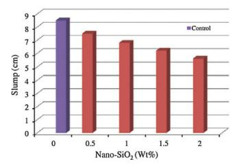
Figure 4. The influence of NS on the workability of concrete [86].
