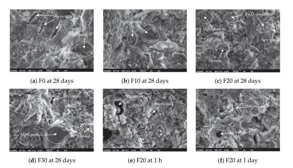
Figure 14. SEM images of MPC pastes with several dosages of Fe<sub>2</sub>O<sub>3</sub> powder [28].
