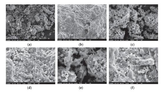
**Figure 17.** SEM images: (**a**,**c**,**e**) for NF-30; (**b**,**d**,**f**) for NF-90 [28].
