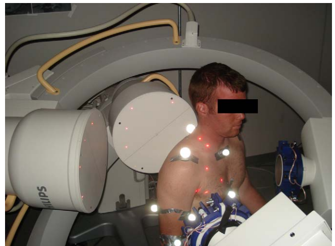
Figure 2. The biplane fluoroscopy system consisting of 2 synchronized C-arms with the subject's shoulder positioned in the 3-dimensional viewing area.
