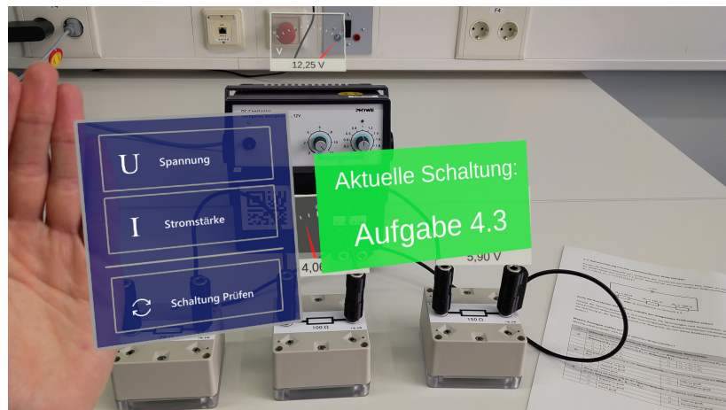
Figure 9. Screenshot of the menu attached to the hand of the participant. The visible options are Spannung (voltage), Stromstärke (current), and Schaltung prüfen (check circuit). As the participant has just checked the circuit, the green window indicates a valid circuit and displays Aufgabe 4.3 (task 4.3) to confirm the task matching the current circuit setup.
