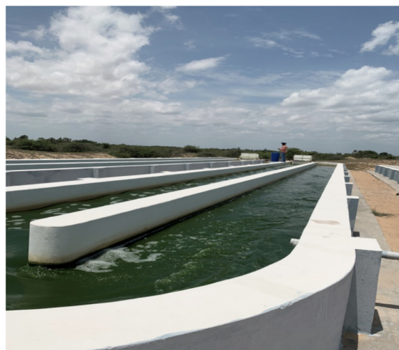
Fig. 1. Outdoor mass culture of marine Chlorella vulgaris (NIOT-74) in 25 ton raceway ponds.
