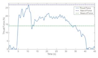
Fig. 3: The force variation when the drill approaches the bone and passed through the proximal cortex – medulla – distal cortex (Drill 3).
