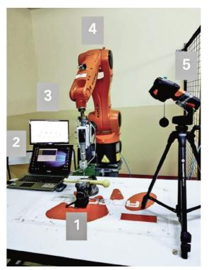
Fig. 2: Experimental setup: (1) Compressed humerus sawbone [Synbone®, Swiss] in a clamp. (2) Computer where data and measurements are saved. (3) Drill attachment, measuring sensors and drill. (4) Robotic arm [Kuka Kr900®, Kuka Roboter GMBH]. (5) Thermal camera [Testo 869®].
