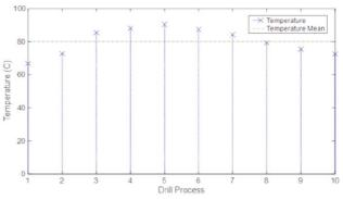
Fig. 6: Temperature variation of the drill bit during drilling measured with a thermal camera (Drill 1). Each temperature measurement was made as the drill process was finished for each hole before beginning the next hole.
