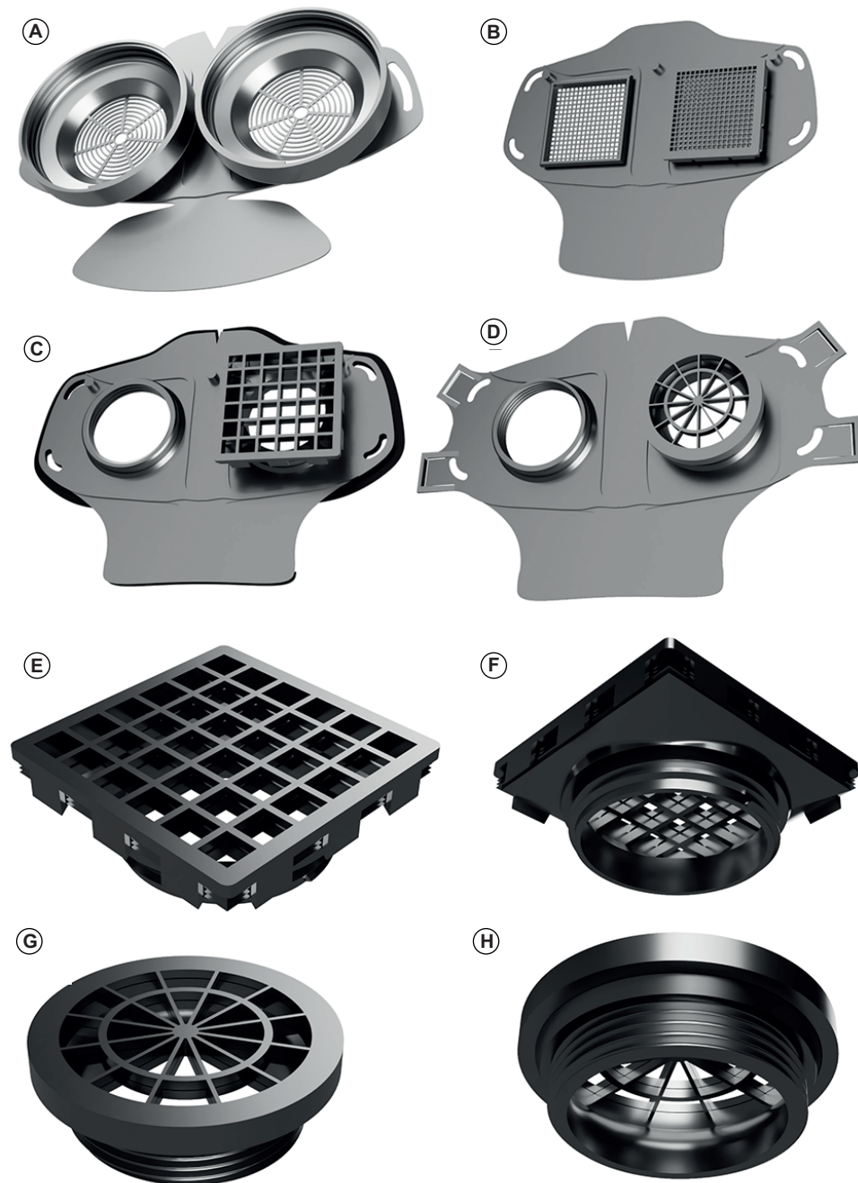
Figure 2. Mask design variants of the HSU/BwKWST face masks. Four different variants of the HSU/BwKWST face masks were produced. The HSU/BwKWST FM V1 is shown in (A). (B) depicts the HSU/BwKWST FM V2 with a new mask design at the chin area, fixation pins for an additional face shield and altered fixation holes for elastic bands. (C) HSU/BwKWST FM V3 with an additional inlay made from black TPU95A (black rim) and a novel design of the nasal cut. (D) shows the further developed HSU/BwKWST FM V4 with four fastening strips and without the TPU inlay that was previously incorporated to V3. (E) and (F) show the square filter design with a clip fastening mechanism and (G) and (H) the round filter design with a fastening thread.
