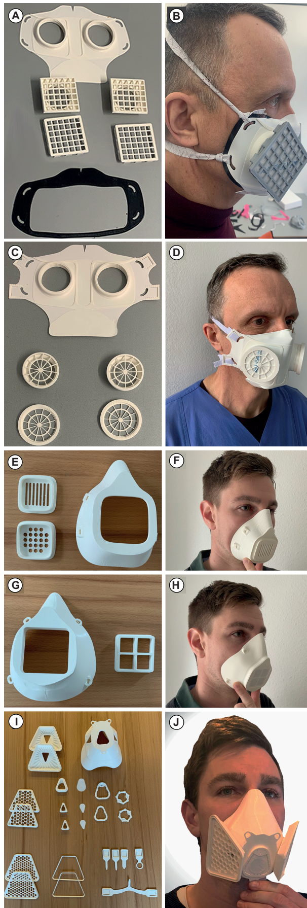
Figure 3. Mask overview. (A) Depiction of the individual parts of the foldable HSU/BwKWST FM V3 made from thermoplastic PLA and the TPU95A inlay. (B) HSU/BwKWST FM V3 test fitted to the experimenters face. (C) Depiction of the individual parts of the foldable HSU/BwKWST FM V4 made from thermoplastic PLA. (D) HSU/BwKWST FM V4 test fitted to the experimenters face. (E) The individual parts of the COVID-19 Mask V2 made from PLA are shown. (F) The COVID-19 Mask V2 test fitted to the experimenters face. A picture of the COVID-19 Mask V2 made from TPU95A is not provided, as it would not provide additional information. (G) Image of the parts of the Montana Mask. (H) The Montana Mask fitted to the researchers face. (I) The individual parts of the Maker Mask are presented with the mask being test fitted in (J).
