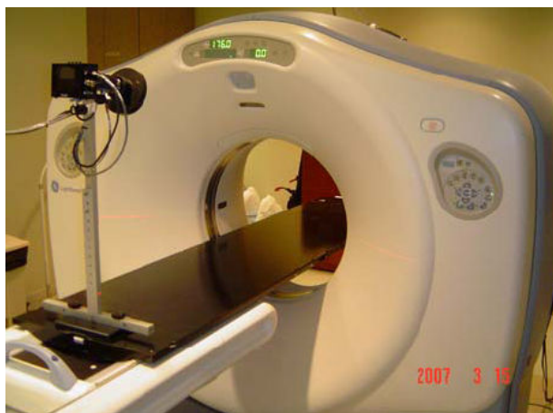
Figure 3 The location of the infrared camera at the foot of the couch for tracking the marker block in the RPM system.
