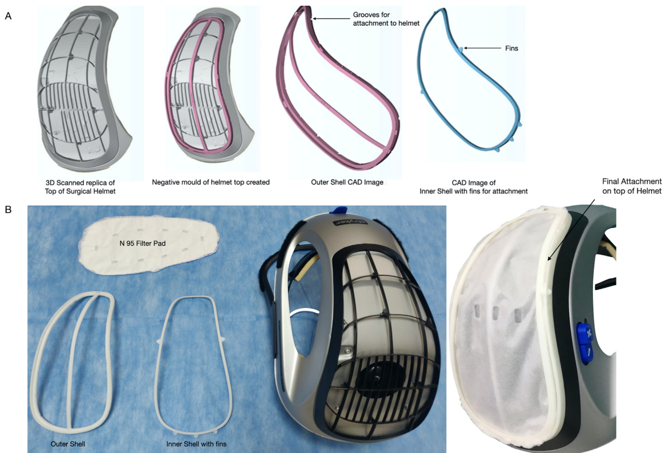
Fig. 4. CAD-CAM design of 3D printed template (A) and Helmet construct (B).
