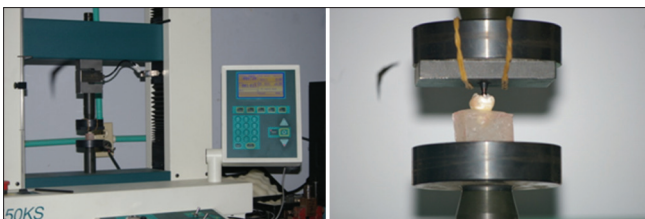
Figure 6: Application of physical compression tests on a universal testing machine (Tinius Olsen® H50KS)
