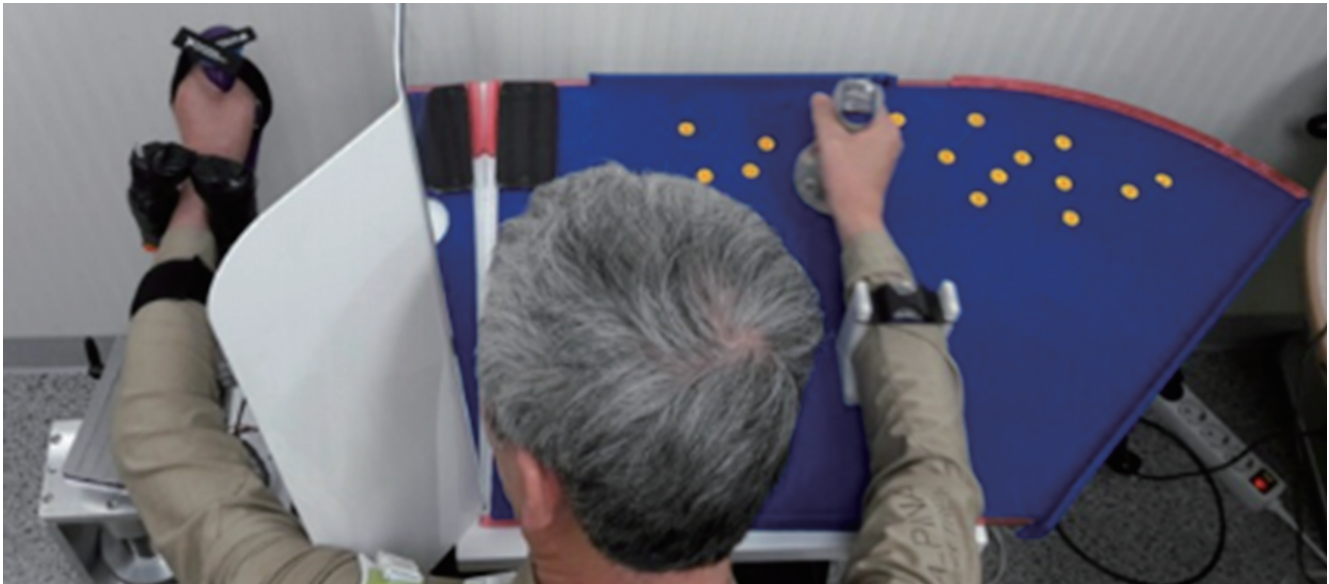
Fig. 1. A 56-year-old male chronic stroke patient is performing the robotic mirror therapy by moving his intact (right) arm while the hemiplegic (left) arm is moved by the 2-axis robot symmetrically.
