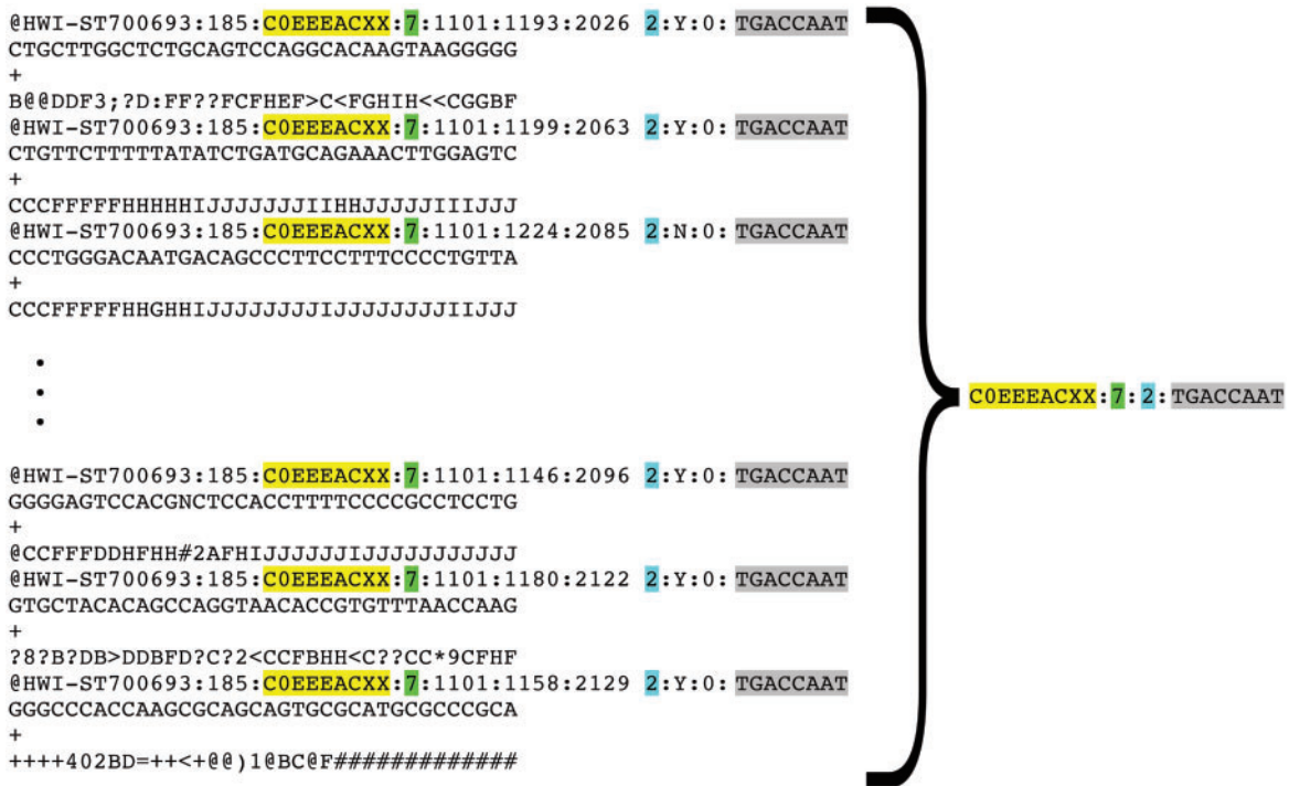
Figure 5. Representation of FASTQ file content by FASTQ signature. FASTQ signature is constructed using read name parts that are common for multiple reads within a single FASTQ file. Read name parts that are used for signature construction are color coded in the figure: flowcell identifier (yellow), flowcell lane number (green), read 1 or read 2 (turquoise) and index sequence (grey). Our condensation approach allows representation of multiple reads in FASTQ file by a single FASTQ signature, as it is exemplified in the figure.
