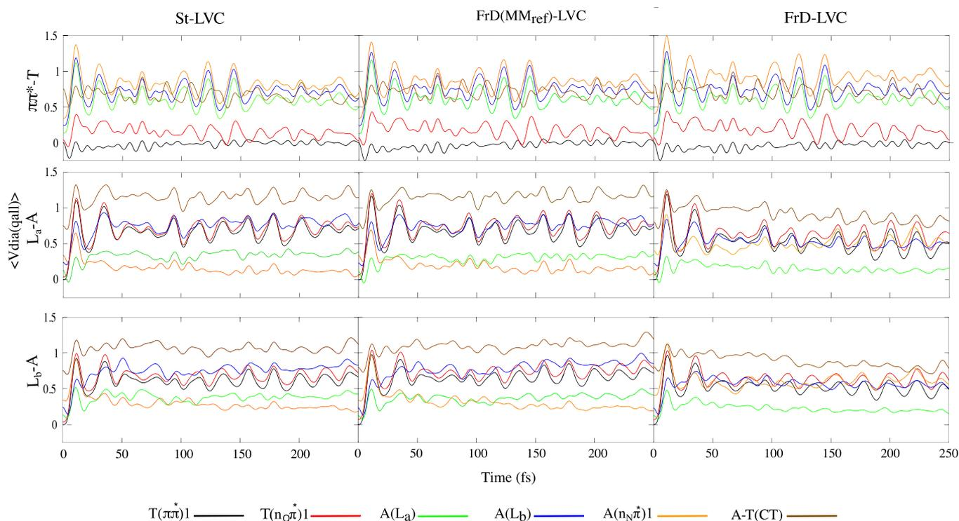
**Figure 5.** Expectation of diabatic PES for AT with initial excitation of  $T(\pi\pi^*1)$  (top),  $A(L_a)$  (middle), and  $A(L_b)$  (bottom) obtained by St-LVC (left), FrD( $MM_{ref}$ )-LVC (middle), and FrD-LVC (right). For clarity, only the first six diabatic states are shown. The full figure is shown in Figure S9 in the SI.
