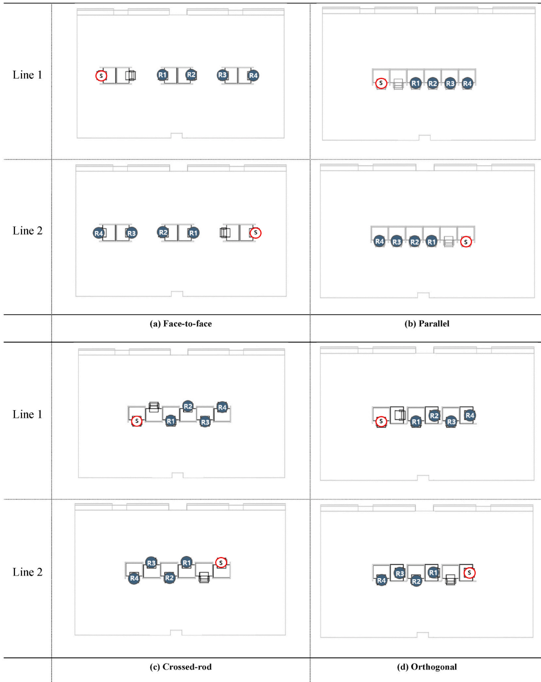
Fig. 2. Locations of sound sources and receiving points for different layouts: (a) face-to-face, (b) parallel, (c) crossed-rod, and (d) orthogonal.
