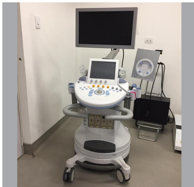
Figure 1. Ultrasound device with elastography imaging activation mode. Aixplorer, v9 (Supersonic Shearwave Imaging, Aix-in-Provence, France). Source: photo archive of the service.
