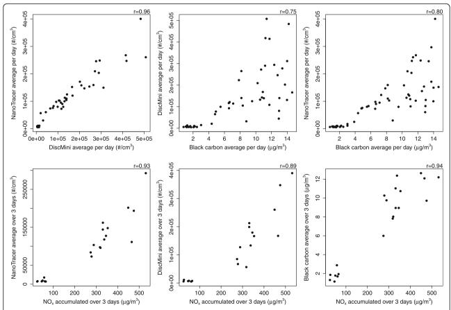
**Fig. 1** Correlation between air pollution components in diesel and electric trains. The data corresponds to 63 (UFP and black carbon measured with NanoTracer equipment and Aethalometer, respectively) and 55 (UFP measured with DiscMini equipment) days of exposure. Nitrogen oxides were measured over 3 days, corresponding to 18 periods
