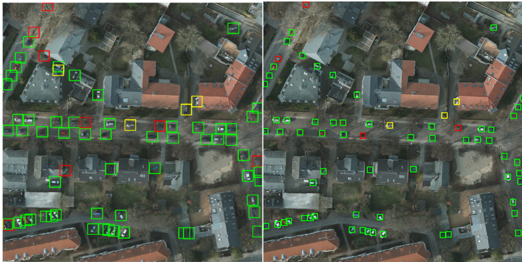
Figure 12. Visual comparison between the detection model obtained by the NATO Innovation Challenge winning team (left-hand side) and our detection model (right-hand side).
