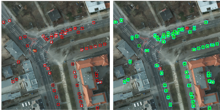
Figure 4. Objects considered for training (marked with green border) and ignored objects (red border). On the left-hand side, the anchors have default dimensions, while on the right-hand side they are optimized.
