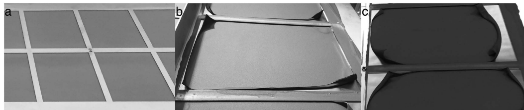
Figure 1. (a) Sample A coated onto graphite foil. The only visible difference among samples A, B and C was a slight difference in color, in which samples B and C were a slightly darker shade of gray. (b) Sample D coated onto graphite foil with some shrinkage and deformation effects at the edges of the electrode. (c) Sample E coated onto graphite foil with large shrinkage and deformation at the edges and along the sides of the electrode.
