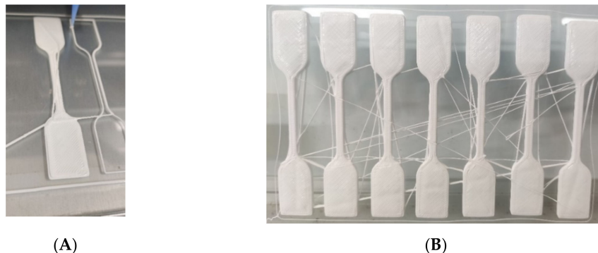
Figure 3. The photos of (A) printing the first layer of the dumbbell specimen; (B) the cured dumbbell specimens in one combination group.
