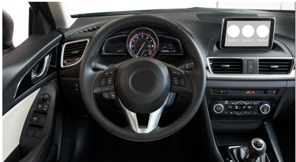
Figure 2. SSVEP-based driving mode selection system: a view of the car dashboard and the SSVEP interface in the middle.
