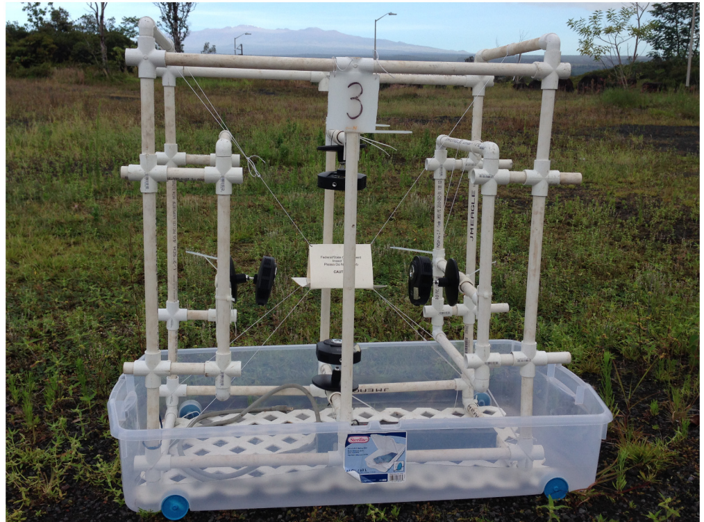
Fig 1. Apparatus for image capture and fly detection 5 surfaces of a Jackson trap. Four cameras were used to image two internal surfaces, both top surfaces and the bottom of the trap. We did not image the sticky panel at the bottom of the internal area. The tub used to collect flies that dies without being captured on the sticky panel is also pictured.
