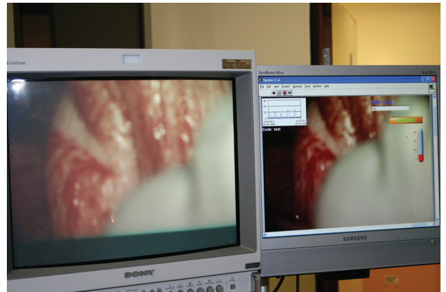
Figure 2. Graphic output of force versus time displayed on parallel computer monitor in real time. Also shown on the second monitor are two alternative prototype displays representing the applied force.
