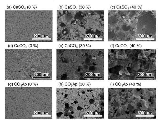
**Figure 1.** SEM images of gypsum (CaSO<sub>4</sub>) blocks ( $\mathbf{a}$ - $\mathbf{c}$ ), CaCO<sub>3</sub> blocks ( $\mathbf{d}$ - $\mathbf{f}$ ), and carbonate apatite (CO<sub>3</sub>Ap) blocks ( $\mathbf{g}$ - $\mathbf{i}$ ).
