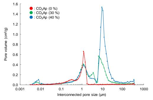
Figure 2. Pore size distribution of CO<sub>3</sub>Ap blocks measured by mercury intrusion porosimetry.
