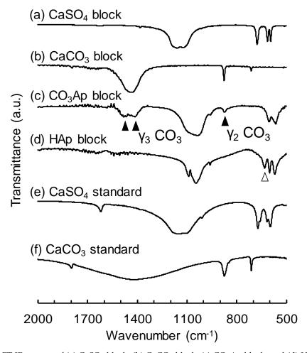
**Figure 4.** FT-IR spectra of (a) CaSO<sub>4</sub> block, (b) CaCO<sub>3</sub> block, (c) CO<sub>3</sub>Ap block, and (d) HAp block compared to X-ray diffraction (XRD) patterns of (e) CO<sub>3</sub>Ap powder and (f) CaCO<sub>3</sub>.
