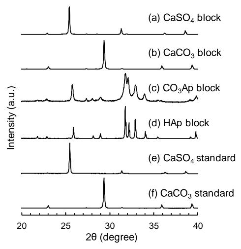
**Figure 3.** XRD patterns of (**a**) CaSO<sub>4</sub> block, (**b**) CaCO<sub>3</sub> block, (**c**) CO<sub>3</sub>Ap block, and (**d**) hydroxyapatite (HAp) block compared to XRD patterns of (**e**) CO<sub>3</sub>Ap powder and (**f**) CaCO<sub>3</sub> block.
