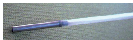
Image 2: OCT probe (Ø 2.7 mm), inserted into the bladder via the working channel of the cystoscope sheath.
