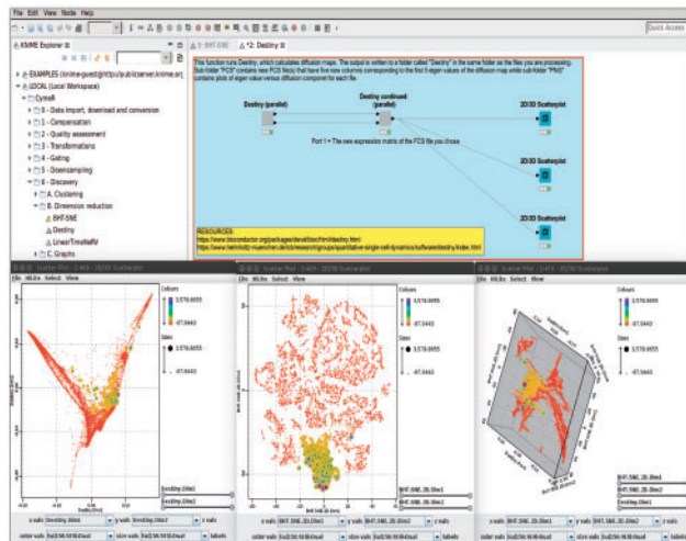
Fig. 1. A screen shot showing the CymeR interface for Destiny on the top and three CymeR scatterplots of the same mass cytometry data colored and sized by a single attribute on the bottom. The bottom-left scatterplot shows the data represented by the first two diffusion components found by the Destiny algorithm while the bottom-center scatterplot shows the data represented by two t-SNE dimensions. The bottom-right scatterplot shows the data represented by the two t-SNE dimensions in the x and y dimensions and by the first diffusion component in the z dimension. The bottom-center scatterplot was also highlighted for cells positive for the chosen attribute, which immediately propagated to all other views of the same data (Color version of this figure is available at Bioinformatics online.)
