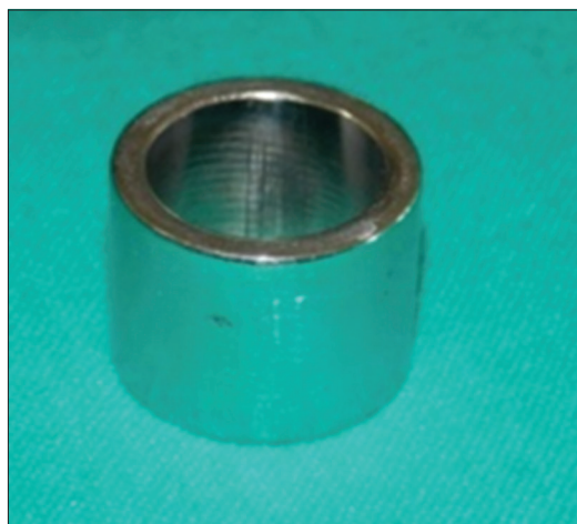
Figure 1: Metallic cylinders (internal diameter 20 mm and height 20 mm).
