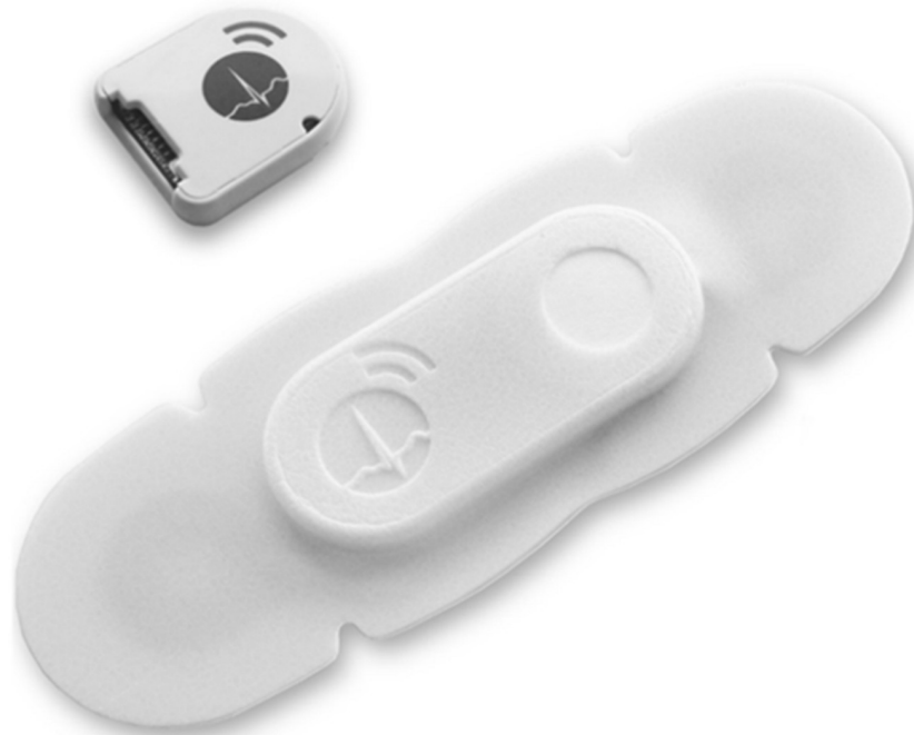
Fig 1. The reusable wireless HealthPatch sensor (left) and disposable HealthPatch (right) [15].
