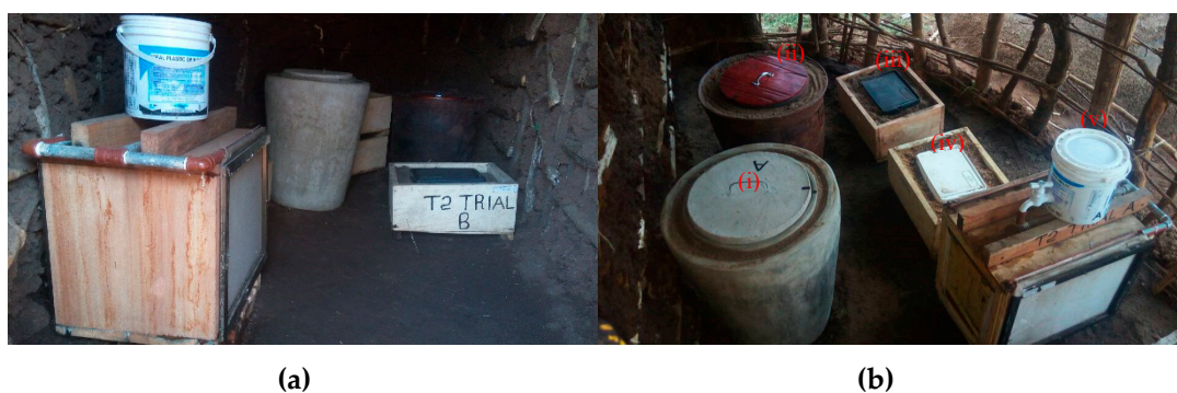
Figure 1. Passive cooling device (PCD) designs stored indoors (a) and outdoors (b). The different PCDs are labeled as follows: (i) Zeepot cementsand, (ii) Zeepot Clay, (iii) Coolbox sand, (iv) Coolbox sawdust and (v) Coolgardie.
