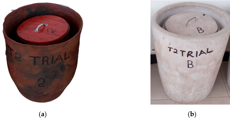
Figure 2. Second generation Zeepot (a) Clay and (b) Cementsand prototypes manufactured and tested during the refinement phase.
