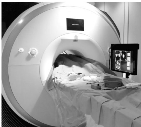
Figure 2 Interventional setup of the magnetic resonance suite using a 3 Tesla magnetic resonance imaging system (Siemens AG, Erlangen, Germany) and a RF-shielded, non-magnetic in-room monitor. Image is adopted from Ref. 50
