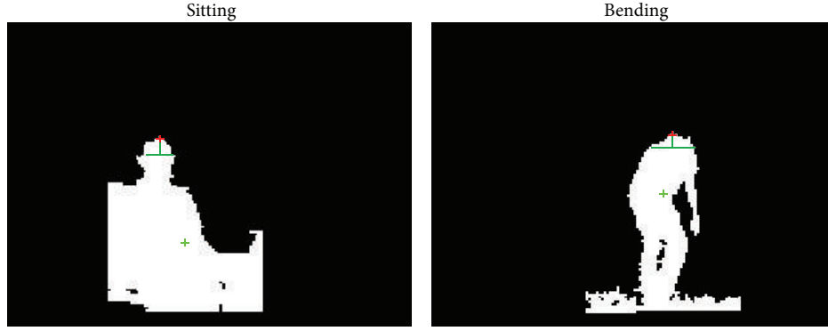
FIGURE 9: Extracted contour region, lines on the top part of the body to calculate the ratio parameter, and tracking point on the extracted region.
